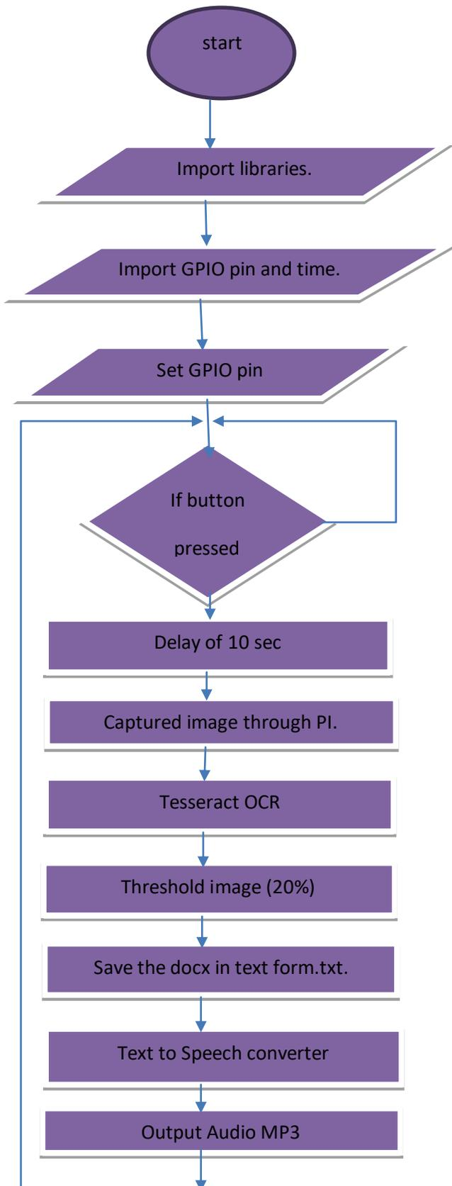
Fig.C suggests the waft chart, all the essential gpio, time and subprocess is imported within the python code, assign gpio pin to push button transfer, if button is pressed after postpone photograph is captured and dispatched to ocr, else it will likely be looping until button is pressed.
